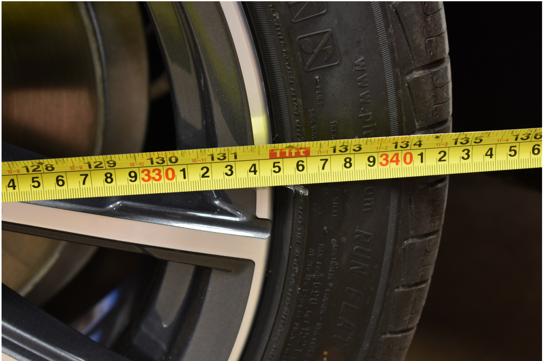
FIGURE 5.25 MEASURING VEHICLE LEFT SIDE WHEELBASE OUTSIDE EDGE TO OUTSIDE EDGE
